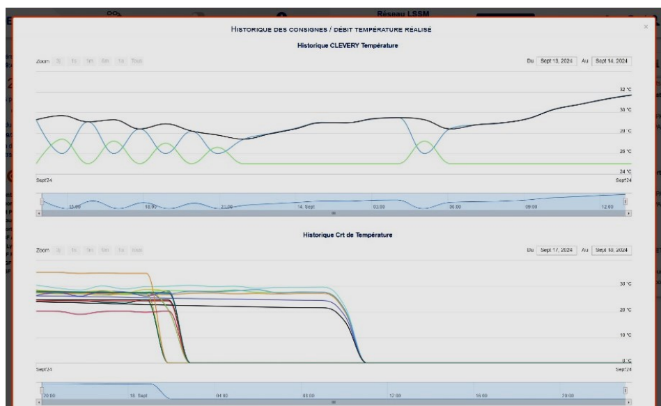
Figure 41: as by the new industrialized temp/flow configuration, in order to follow the loop temperature setpoint sent by Clevery, specific visuals have been integrated to compare sent setpoints, with the values applied on site by the SCADA. Source: DALKIA.
