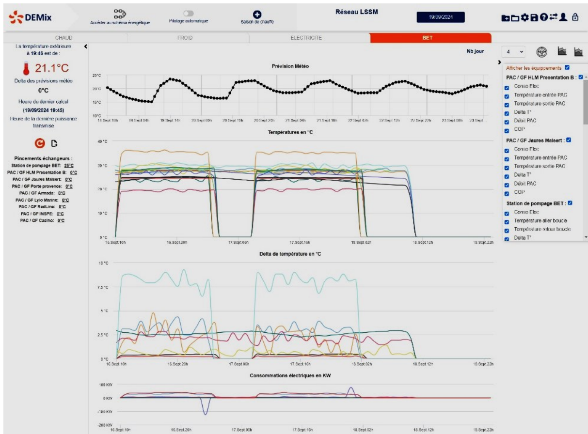
Figure 40 : screen shot of the main hypervision view of the industrialized DEMix platform and adapted the needs of the temp/flow optimisation developments as implemented first in LSSM. Source: DALKIA.
